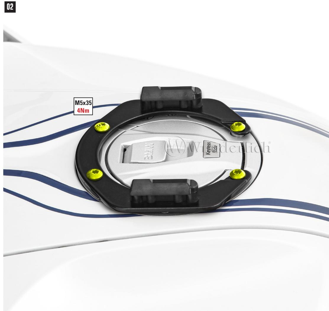
**NACH DER MONTAGE DES TANKRINGES, FUNKTION DES TANKDECKELS PRÜFEN.
