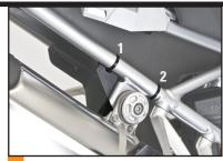
Position the right side wing against the exhaust mount. Install zip ties up from the bottom through the slots, around the frame and in through the outside slots.
