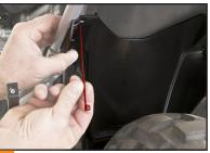
5 Hold the left side wing of the MudSling against the frame. Insert first zip tie up from the bottom through a slot. Zip tie head faces the tire.
