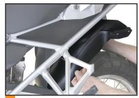
Place MudSling above rear tire and under the existing fender.
