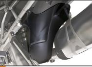
Position the MudSling "shoe" below the existing fender & pull up to engage it.
