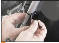
Loop the zip tie around the frame and back in through the slot on the outside. Pull zip tie tight. Install second zip tie.
