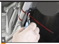
9 Cut off excess zip tie length with a wire cutter for best appearance.
