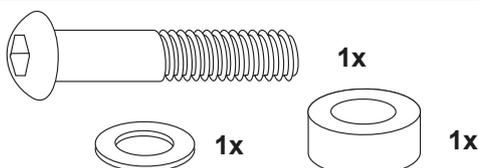
Drehmoment/Torque 38 NM
