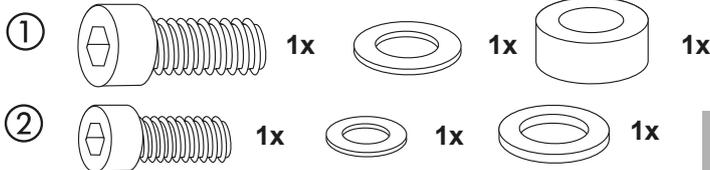
Drehmoment/Torque 19 NM
