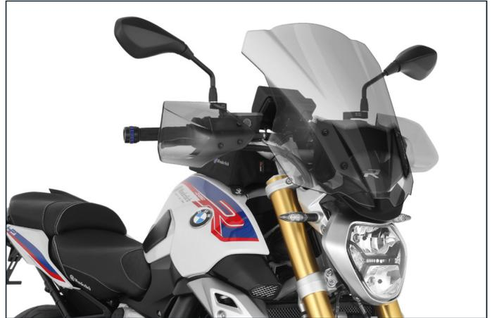
5 mm thick PMMA acrylic plastic, hand polished, no extra edge protection necessary
