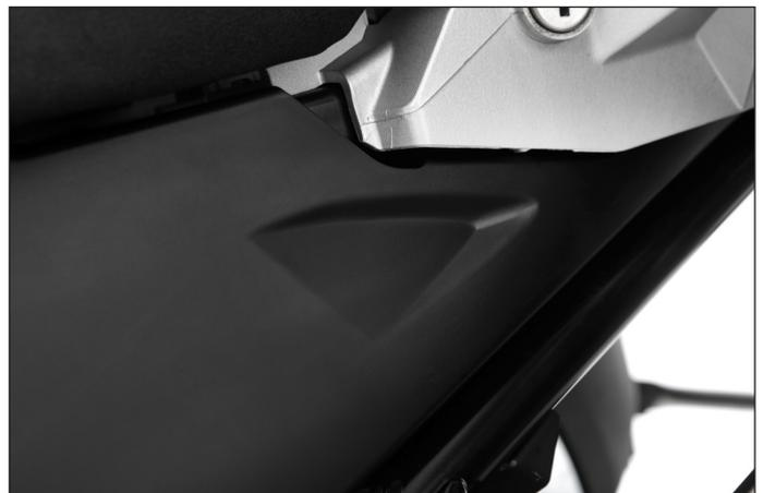
Stability and component rigidity: High-quality PP plastic - with 3 mm component thickness generously dimensioned
