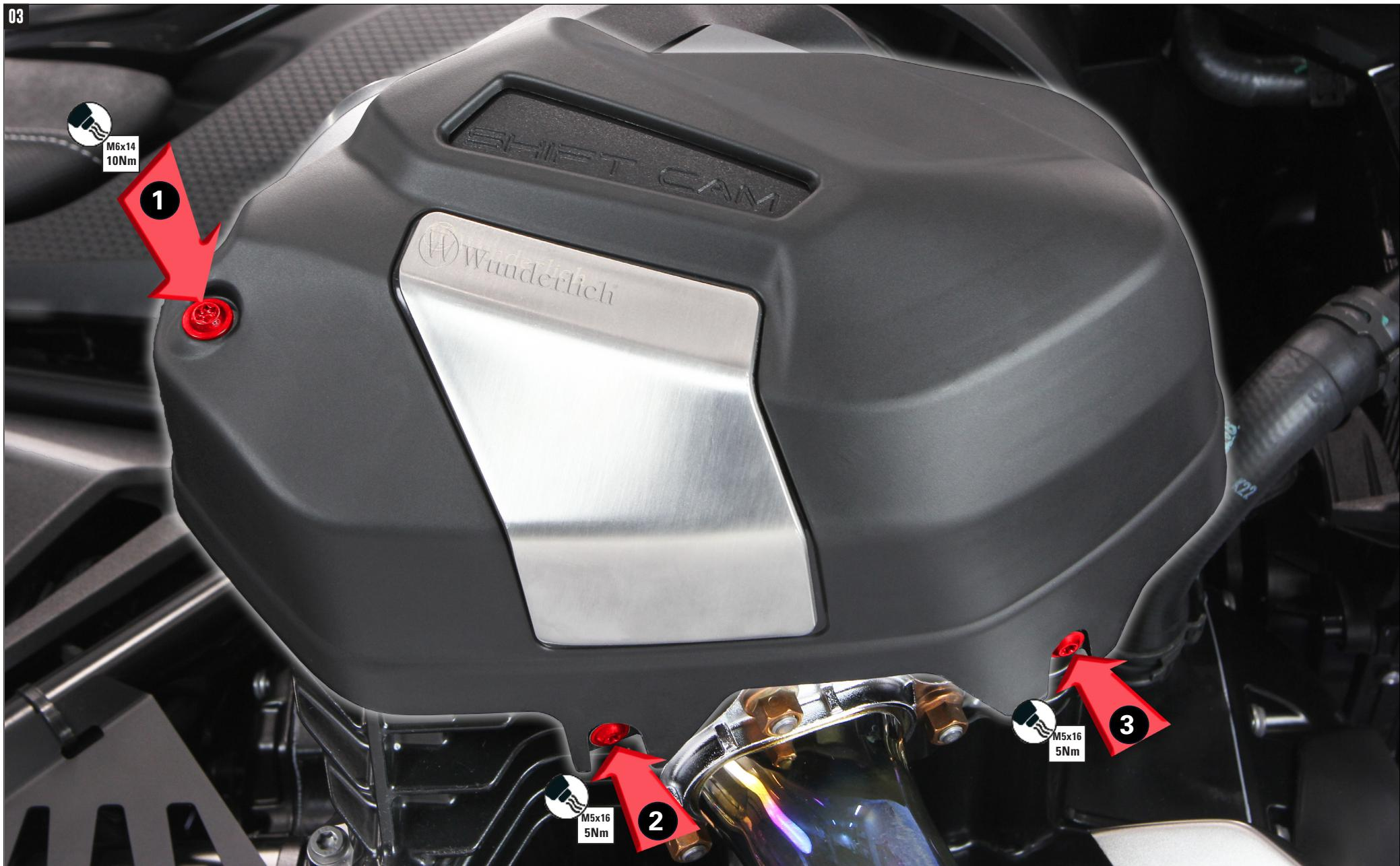
**SCHRAUBEN DER REIHE NACH VORMONTIEREN UND DANACH MIT ANGEgebenEN DREHMOMENT ANZIEHEN.***Pre-assemble the screws in sequence and then tighten to specified torque.*
